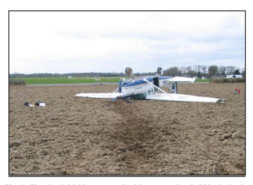
Photo No. 1: Showing initial impact mark with runway threshold in the background
